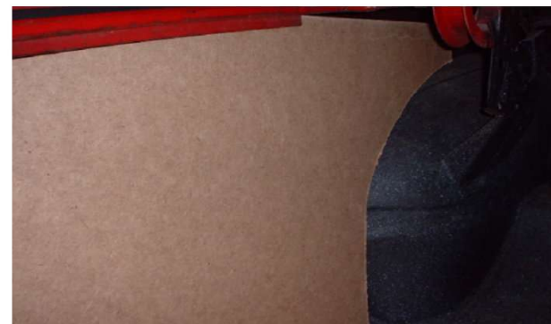
On the left side move the panel back against the light housing for a better fit.
