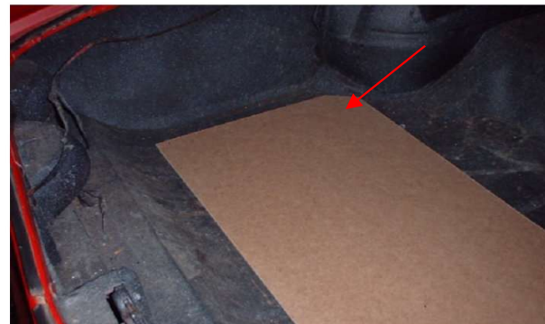
On the left side move the panel back against the upslope of the trunk, note the arrow.
