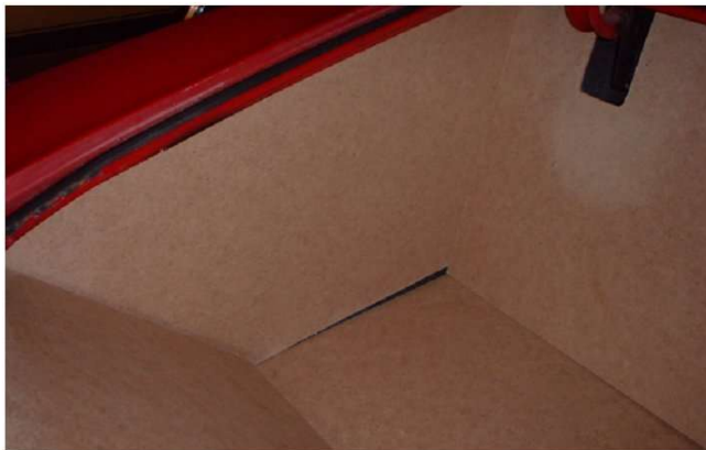
Now all 5 panel pieces are in place ready to upholster with your choice of material.
