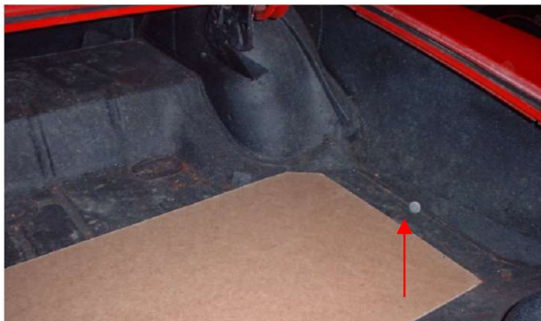
The first panel in fits right up to the jack hold down on the right side of the trunk. Note the arrow with panel in front of the hold down bracket.
