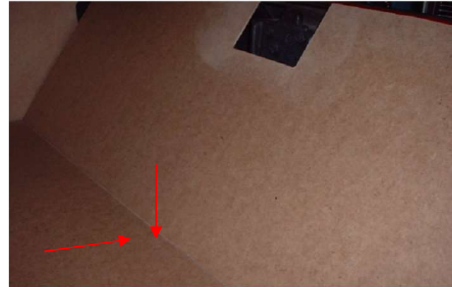
The back trunk latch panel will fit against the two side panels as shown in the pictures. It has a tilt to it and rests on the edge of the floor panel.
