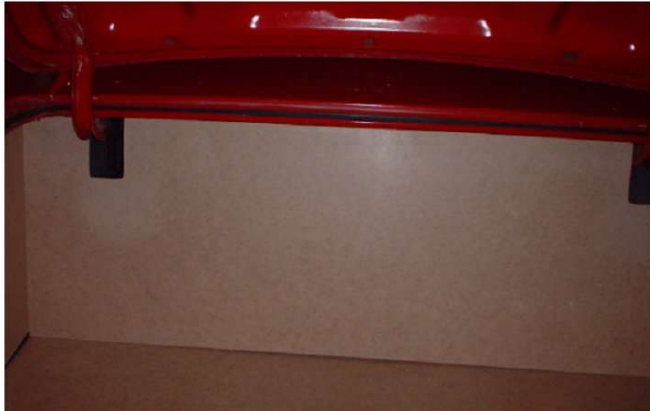
Next is the backside panel, slide this panel in top first with a tilt toward the rear of the trunk.
