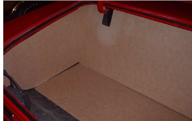
The back panel will fit against the two side panels as shown in the pictures.
